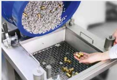
Separating units facilitate separation of mass finished workpieces. Manual separating is time consuming and reduce the efficiency of the process. Automatic separation integrated into mass finishing machine is a great solution for large scale production of small workpieces, which are difficult to be separated manually.
